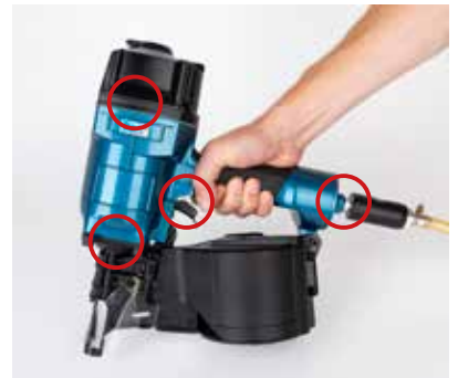
Check for air loss and leaks
