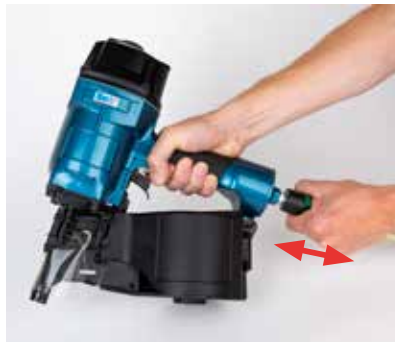
Check condition of air plug nipple and coupling for tightness
