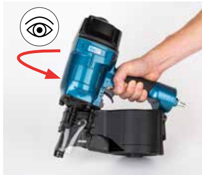
Visual inspection for damage
