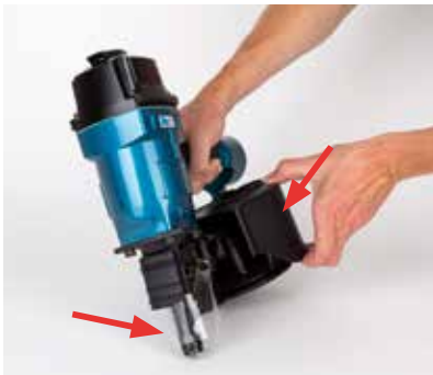
Inspection of the protective and magazine covers
