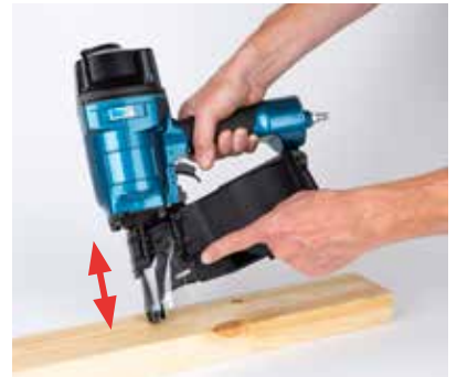
Check for flawless functionality of release mechanism
